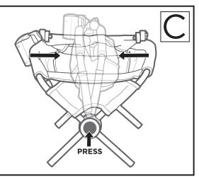
• Press the button on the frame tubes and lift the frame tubes from the hub tubes.
